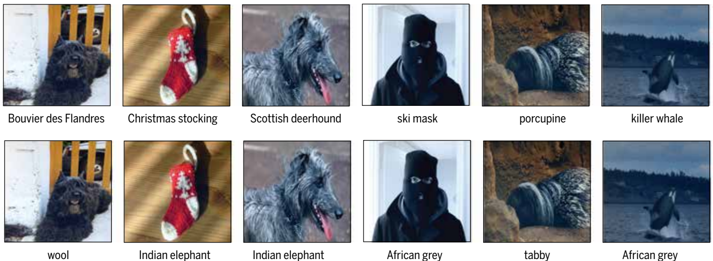
Figure 4. Sample adversarial examples from [20]. The first row shows images and the object that the algorithm recognizes. The second row shows the same images corrupted with noise that is nearly imperceptible, but nevertheless causes the classifier to recognize the wrong object.
